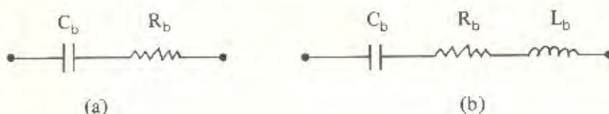
Fig. 5.6 – The Equivalent Circuit of The Human Model
